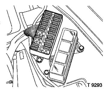
Single fuses are located in the vehicle as follows:
